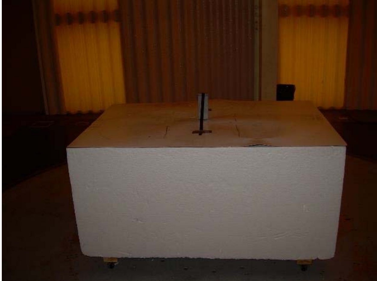
Photograph 1 – Front View of the KP001 Radiated Emission Worst-Case Test Setup
