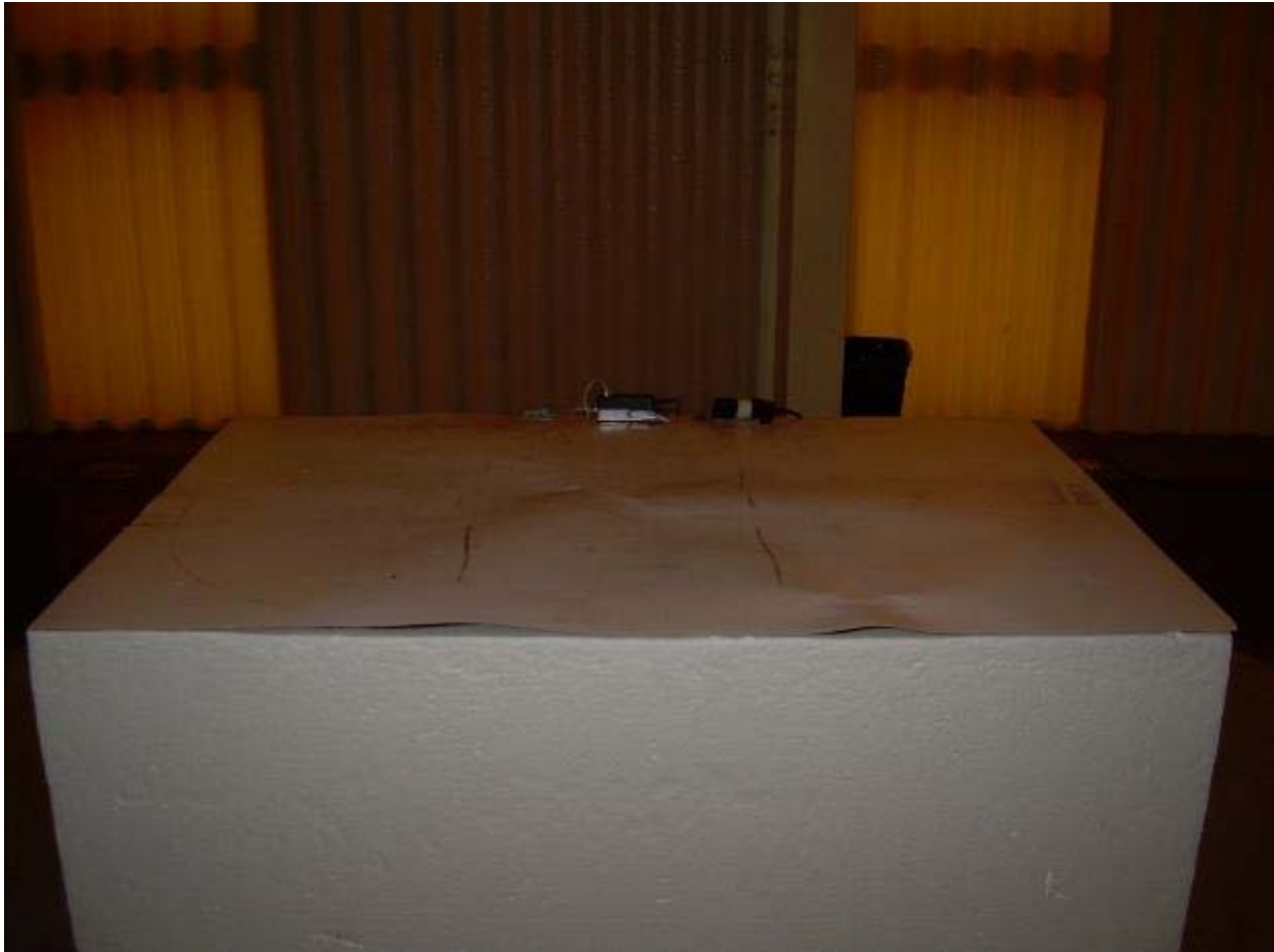
Photograph 5 – Front View of the DS001 Radiated Emission Worst-Case Test Setup
