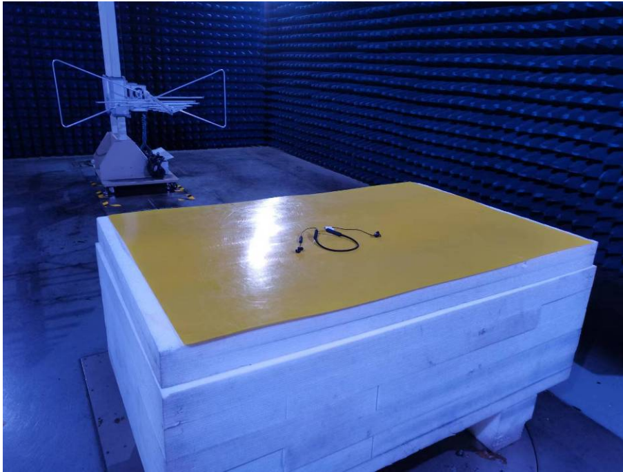
Photo of Radiated Emission Measurement (Above 1G)
