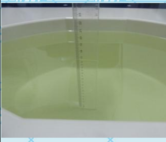
Photo 13: 1800~1900MHz Liquid Depth ≥15.0cm
