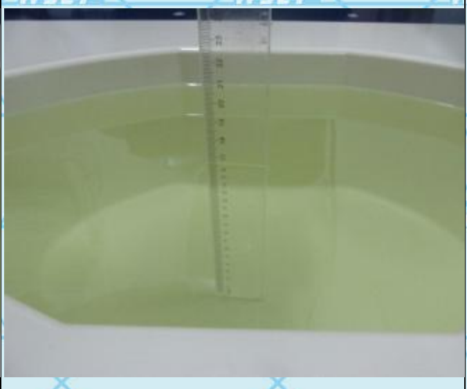
Photo 14: 2450MHz Liquid Depth ≥ 15.0cm
