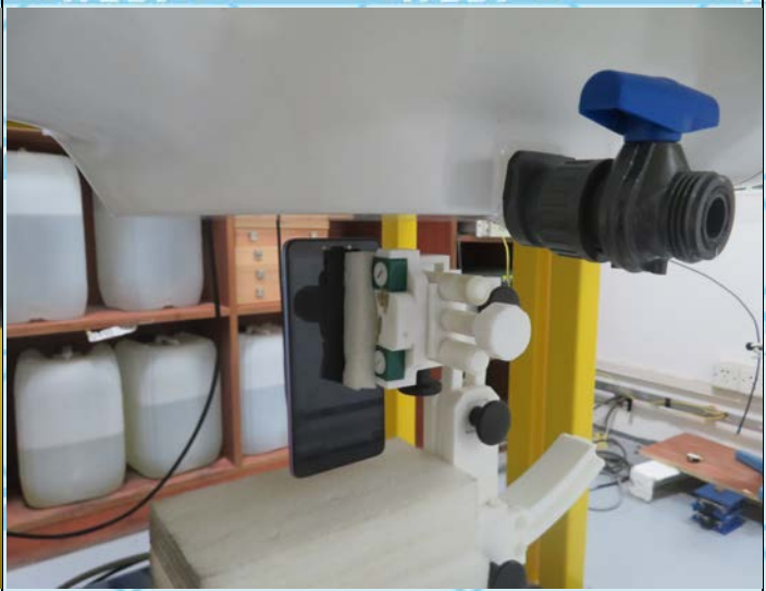
Photo 12: 850MHz Liquid Depth ≥ 15.0cm
