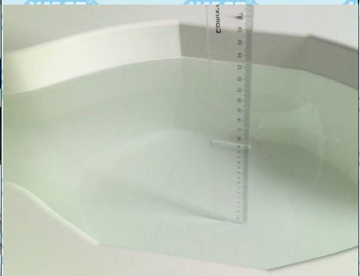
Photo 12: 850MHz Liquid Depth ≥ 15.0cm
