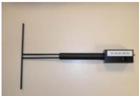
Figure 1 – Satimo COMOSAR Validation Dipole
