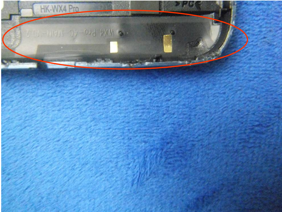
GSM/PCS/UMTS-FDD Antenna View
