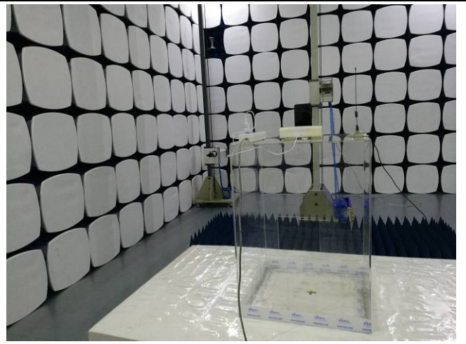
Radiated Spurious Emissions Test Setup Above 1GHz
