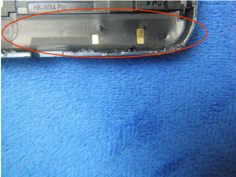
GSM/PCS/UMTS-FDD Antenna View
