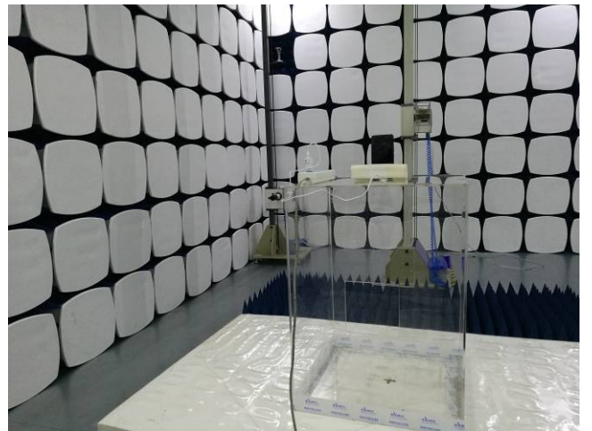
Radiated Spurious Emissions Test Setup Above 1GHz
