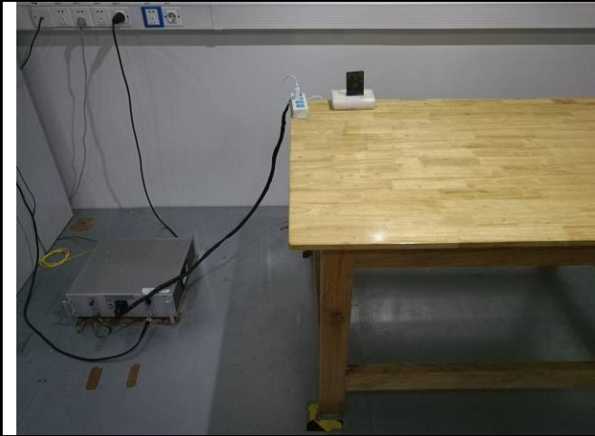
Conducted Emissions Test Setup Front View
