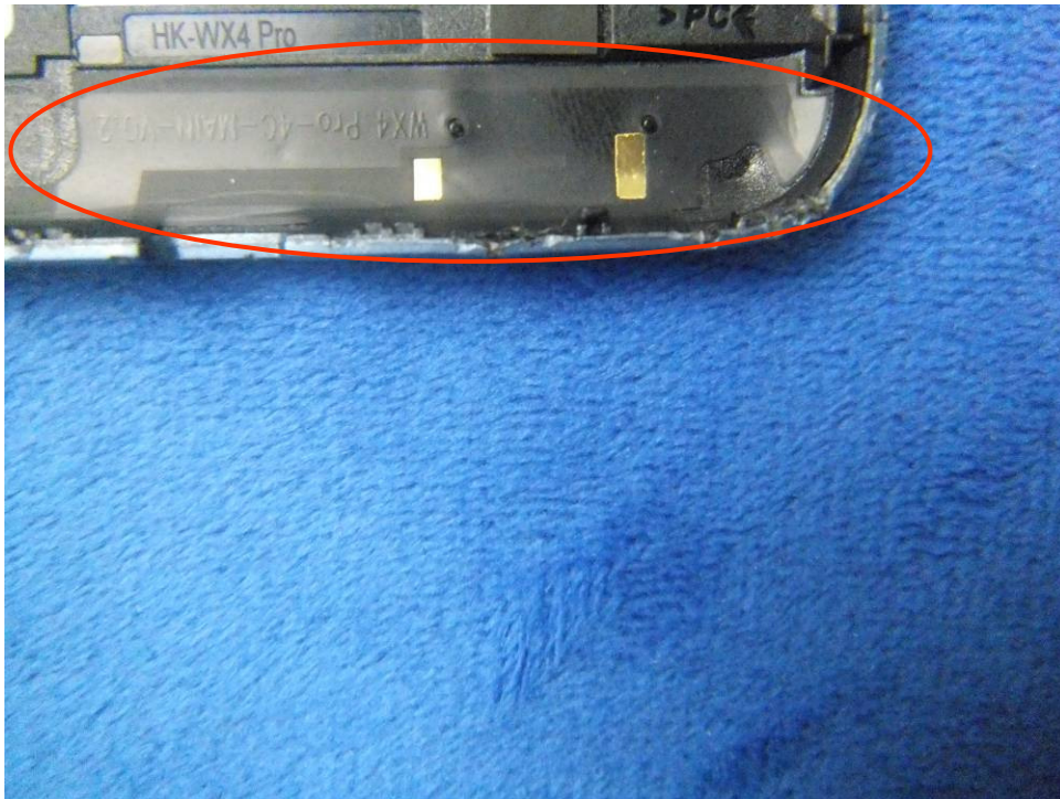
GSM/PCS/UMTS-FDD Antenna View
