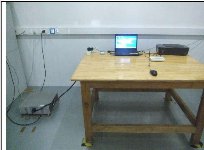
Conducted Emissions Test Setup – Front View
