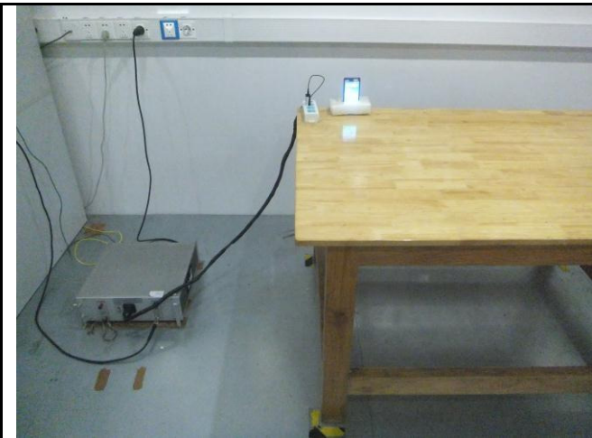
Conducted Emissions Test Setup Front View
