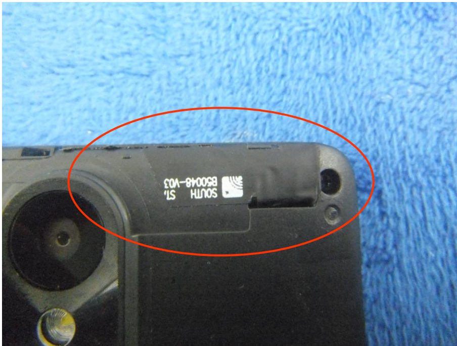
LTE - Antenna View
