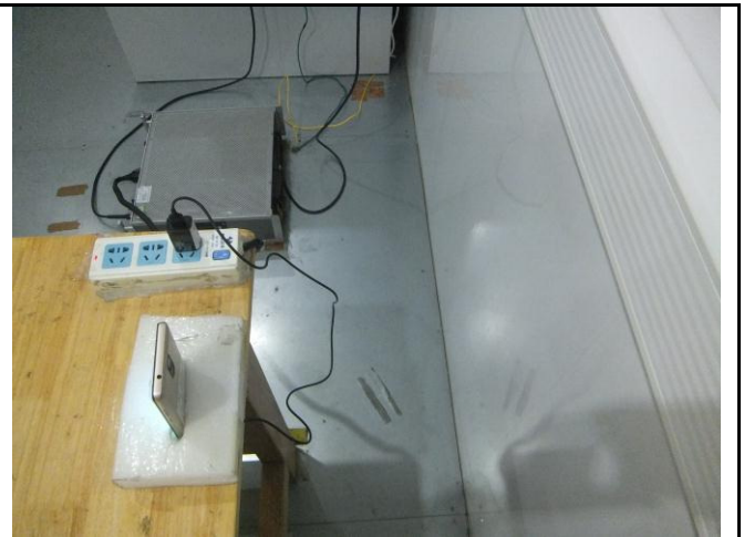
Conducted Emissions Test Setup Side View
