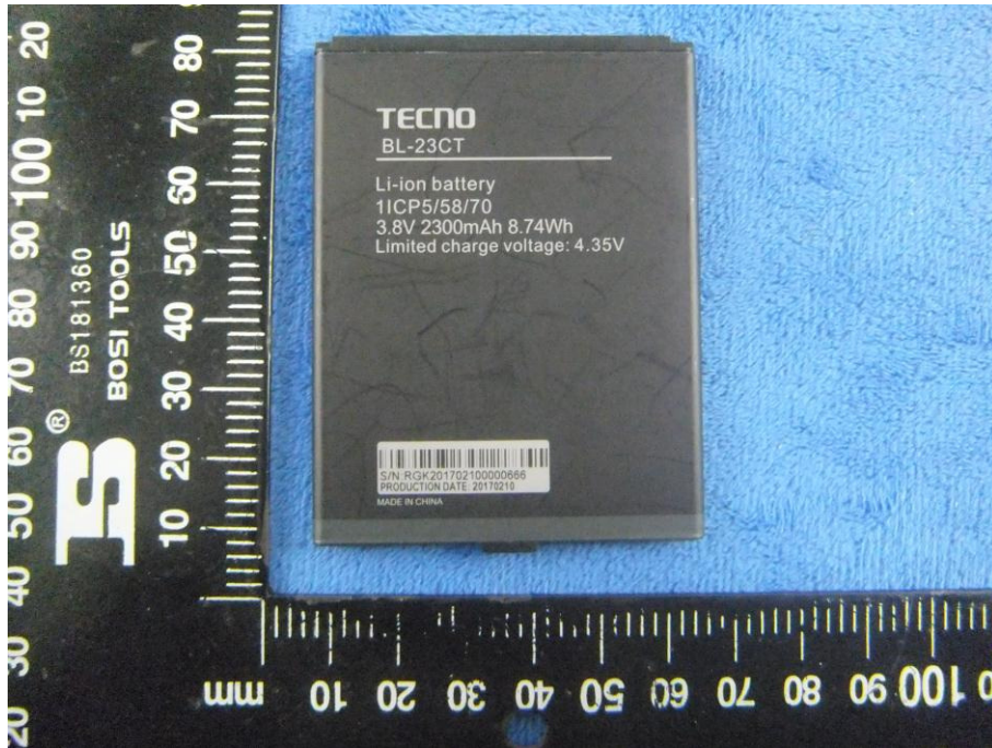
Battery - Front View
