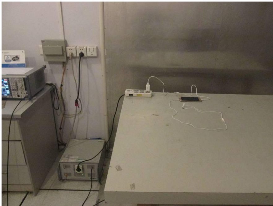
CONDUCTED EMISSION TEST
