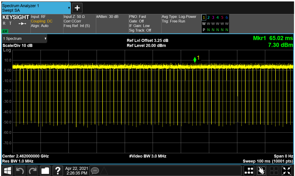
Duty Cycle NVNT n20 2462MHz Ant1
