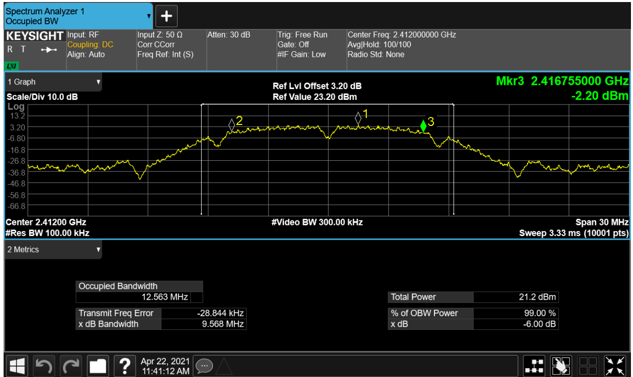
-6dB Bandwidth NVNT b 2412MHz Ant1
