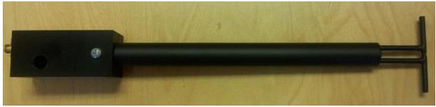
**Figure 1** – *MVG COMOSAR Validation Dipole*
