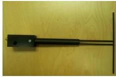
**Figure 1** – *MVG COMOSAR Validation Dipole*
