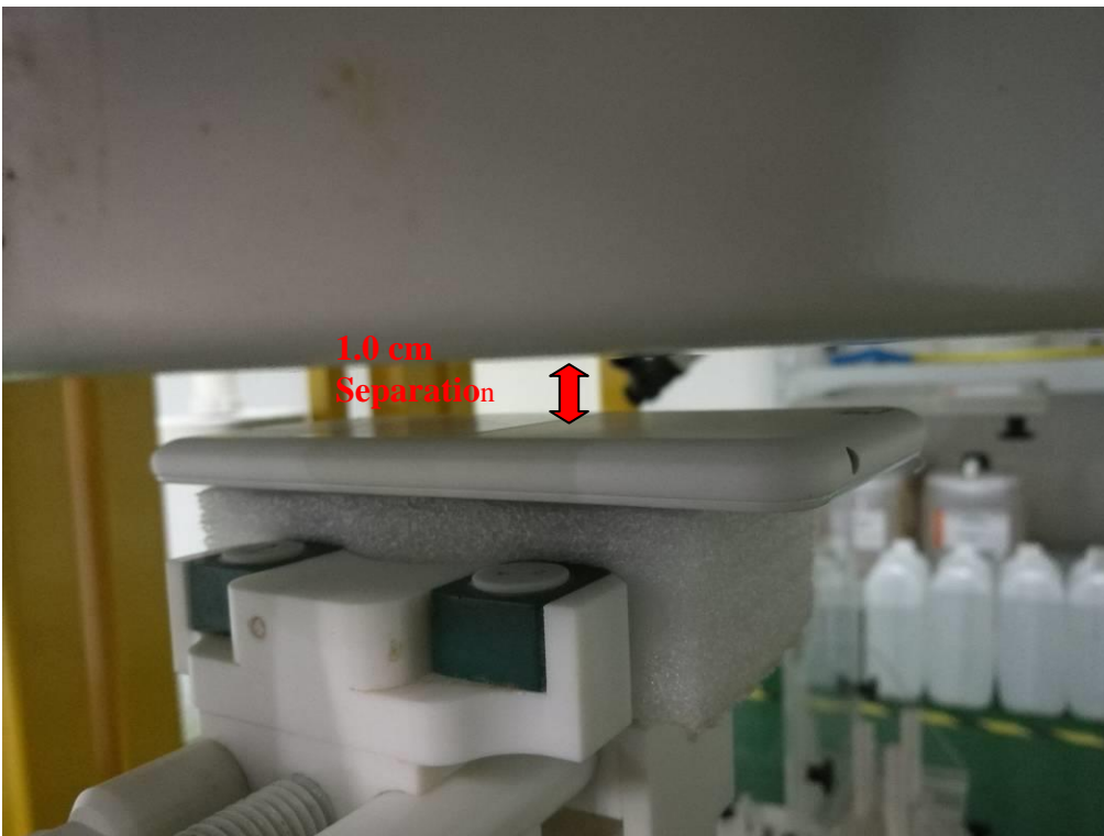
Body Setup Photo (LCD DOWN)
