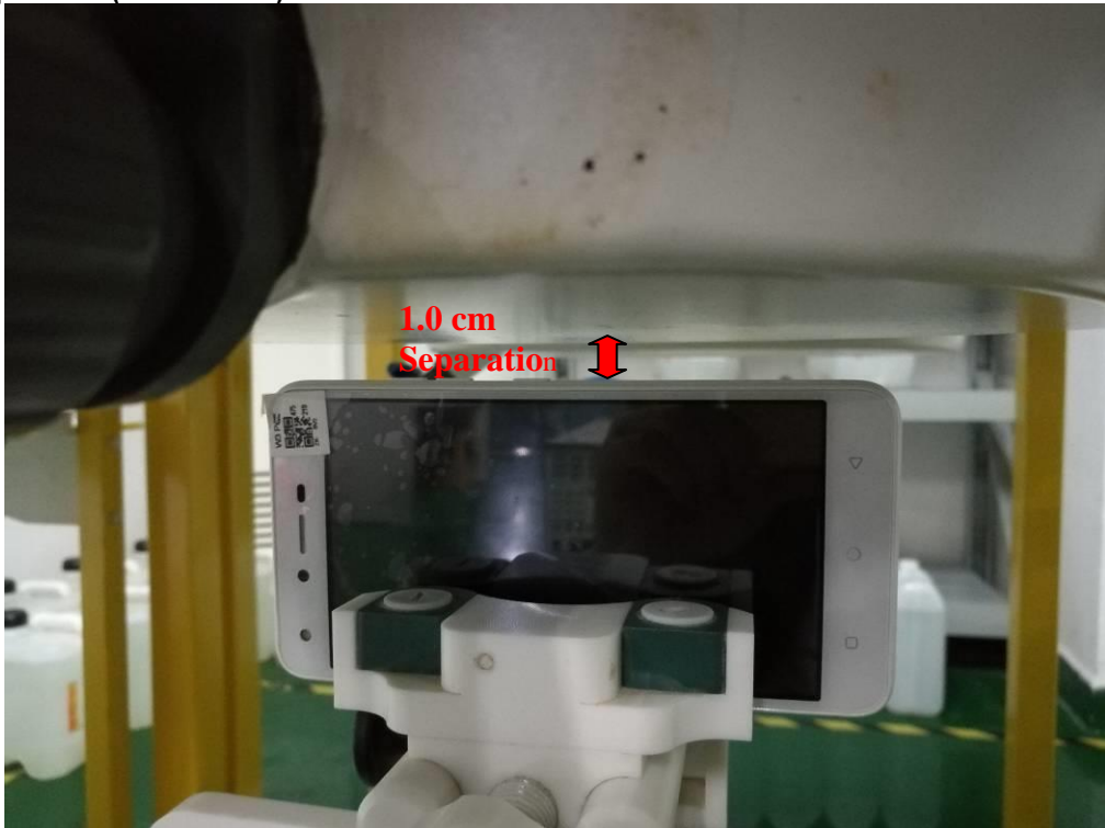
Body Setup Photo (LCD RIGHT)
