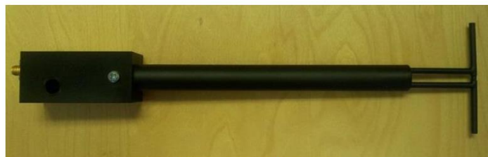
Figure 1 – MVG COMOSAR Validation Dipole
