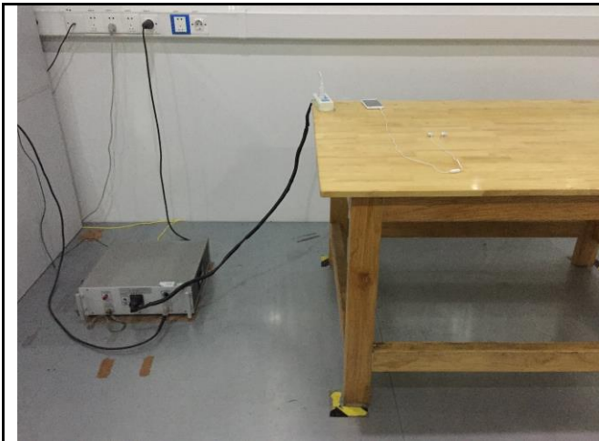
Conducted Emissions Test Setup Front View
