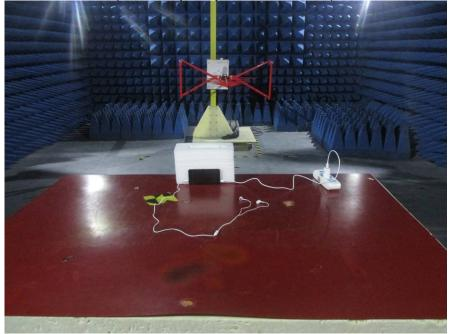
RADIATED EMISSION TEST (Frequency above 1GHz)
