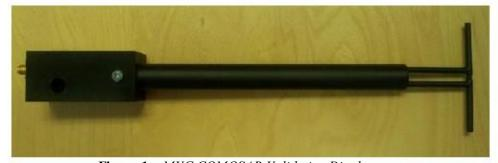
**Figure 1** – *MVG COMOSAR Validation Dipole*
