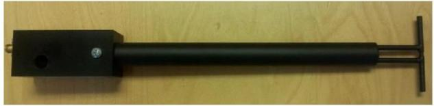
**Figure 1** – MVG COMOSAR Validation Dipole
