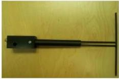
Figure 1 – MVG COMOSAR Validation Dipole
