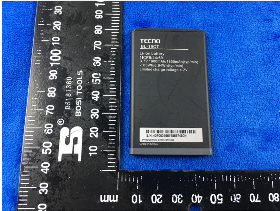
Battery - Front View
