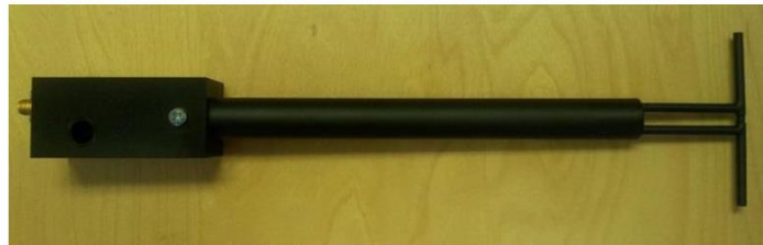
Figure 1 – MVG COMOSAR Validation Dipole
