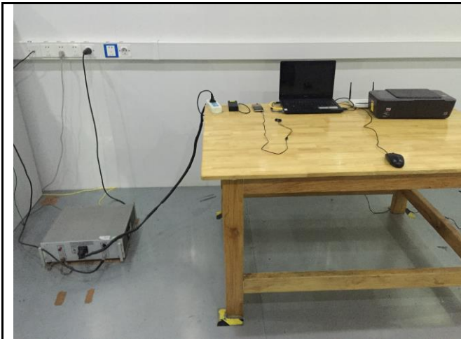
Conducted Emissions Test Setup – Front View
