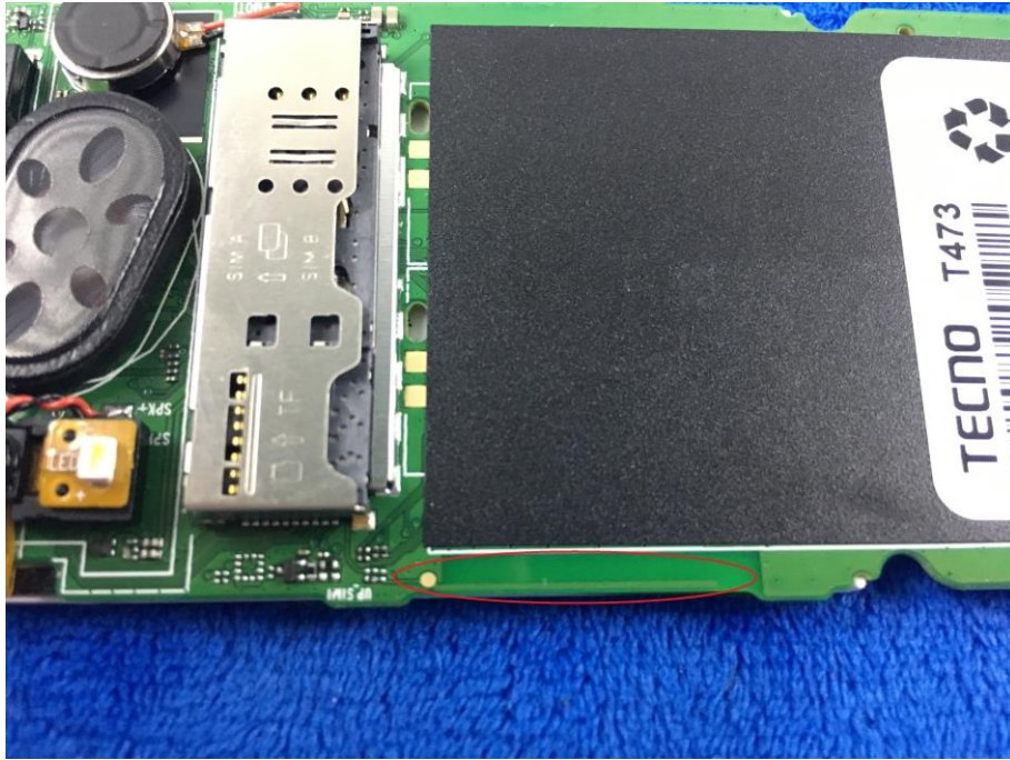
BT - Antenna View
