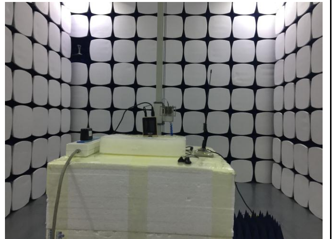
Radiated Spurious Emissions Test Setup Above 1GHz
