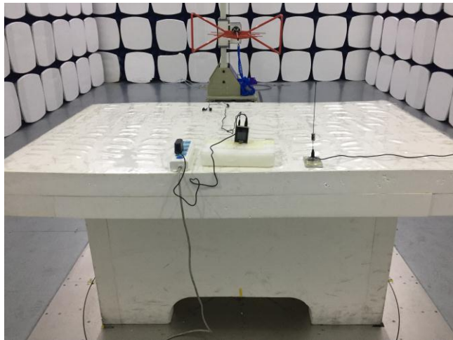
Conducted Emissions Test Setup Front View
