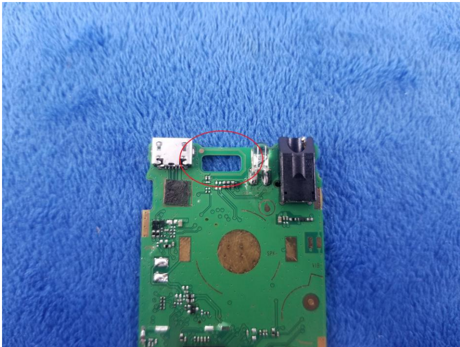
BT - Antenna View
