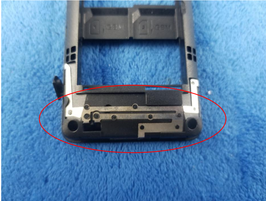
GSM/PCS - Antenna View
