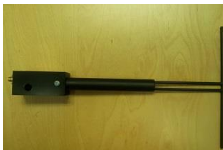
Figure 1 – MVG COMOSAR Validation Dipole
