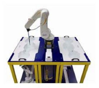
The EUT under test operating at the maximum power level is placed in the phone holder, under the phantom, which is filled with head simulating liquid. The E-Field probe measures the electric field inside the phantom. The OpenSAR software computes the results to give a SAR value in a 1g or 10g mass.
