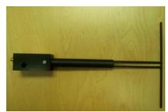
**Figure 1** – *MVG COMOSAR Validation Dipole*
