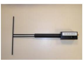
Figure 1 – Satimo COMOSAR Validation Dipole
