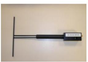
Figure 1 – Satimo COMOSAR Validation Dipole
