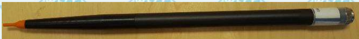
Figure 2 – MVG COMOSAR Dosimetric E field Dipole Dynamicrange:0.01-100W/kg
