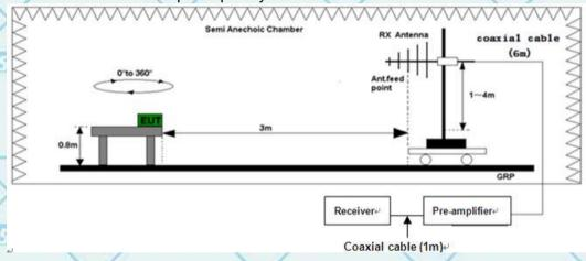
(C) Radiated Emission Test-Up Frequency Above 1GHz
