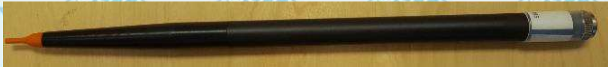
Figure 2 – MVG COMOSAR Dosimetric E field Dipole
