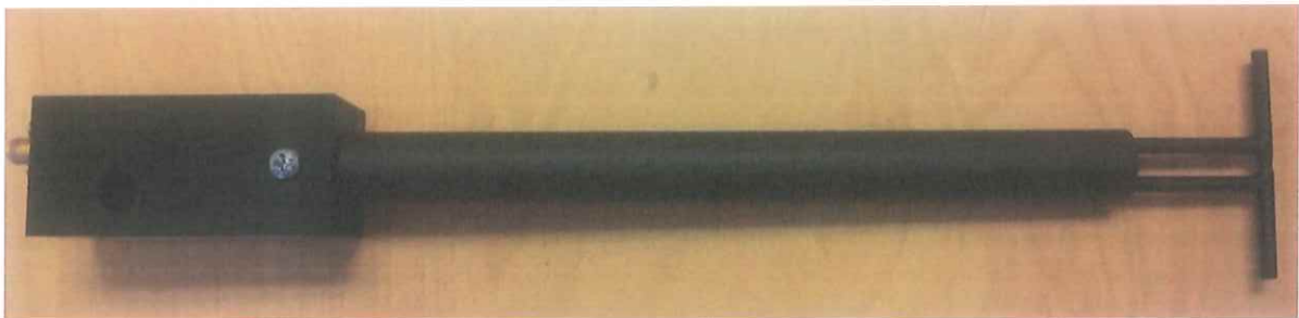
Figure 1 – MVG COMOSAR Validation Dipole
