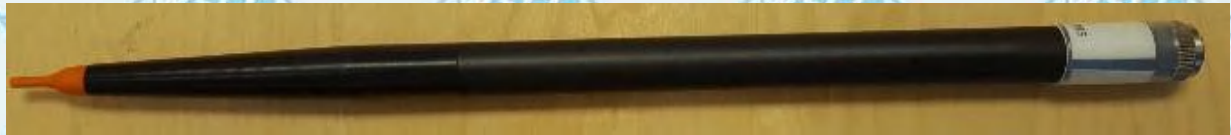
Figure 2 – MVG COMOSAR Dosimetric E field Dipole
