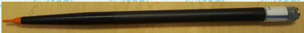
Figure 2 – MVG COMOSAR Dosimetric E field Dipole
