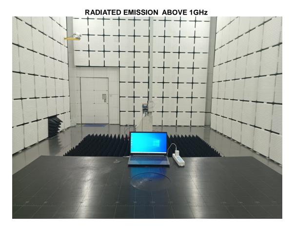
RADIATED EMISSION TEST (Frequency above 1GHz)
