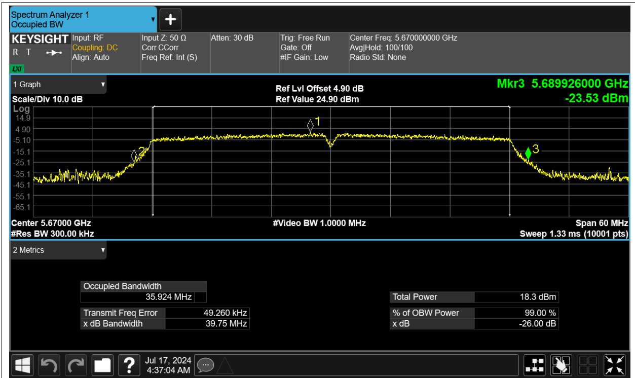
-26dB Bandwidth NVNT ac80 5530MHz Ant1
