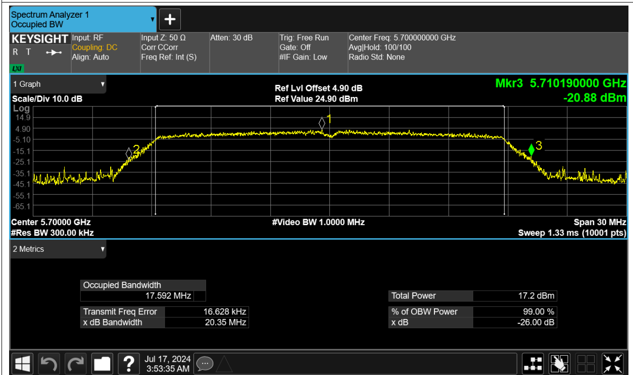
-26dB Bandwidth NVNT ac40 5510MHz Ant1
