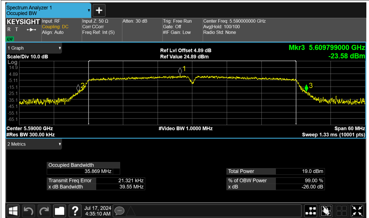
-26dB Bandwidth NVNT ac40 5670MHz Ant1
