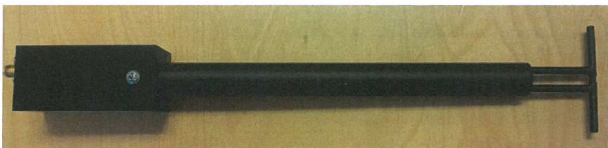
Figure 1 – MVG COMOSAR Validation Dipole
