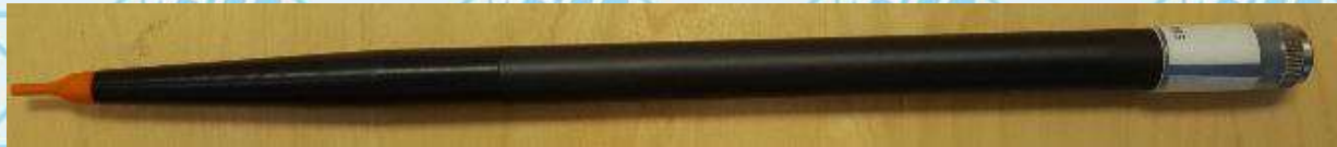
Figure 2 – MVG COMOSAR Dosimetric E field Dipole
