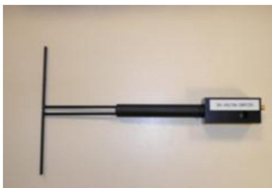
Figure 1 – Satimo COMOSAR Validation Dipole
