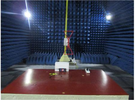
RADIATED EMISSION TEST
