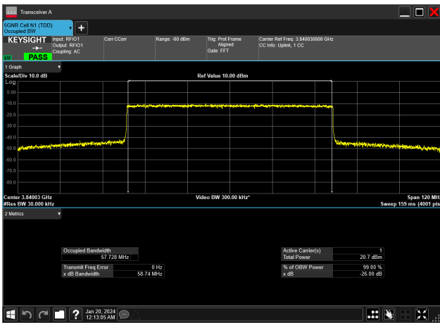
60MHz_30kHz_3840MHz_CP-OFDM 16 QAM_RB162@0&57.728 MHz
