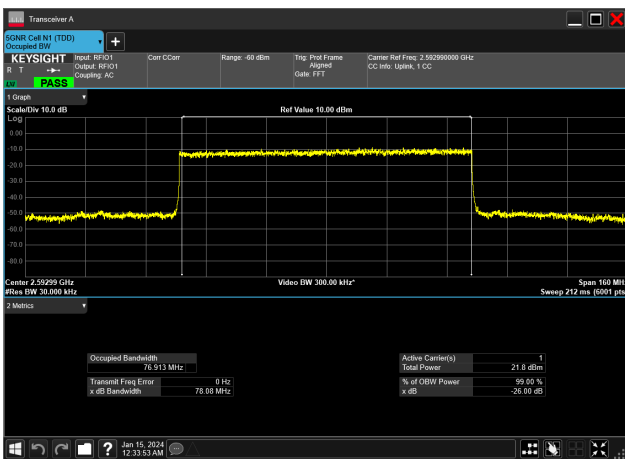
80MHz_30kHz_2592.99MHz_DFT-s-OFDM QPSK_RB216@0&76.913 MHz
