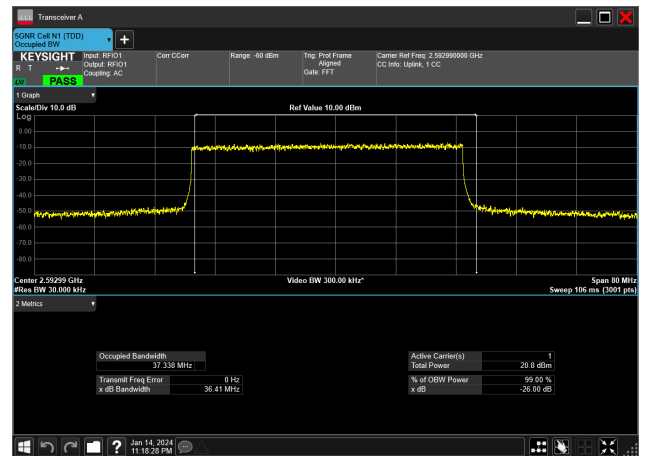
40MHz_30kHz_2592.99MHz_DFT-s-OFDM 16 QAM_RB100@0&amp;37.338 MHz
