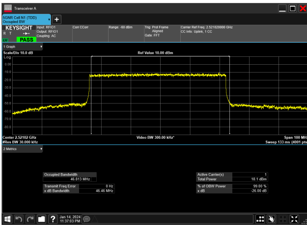
50MHz_30kHz_2521.02MHz_DFT-s-OFDM 256 QAM_RB128@0&46.813 MHz
