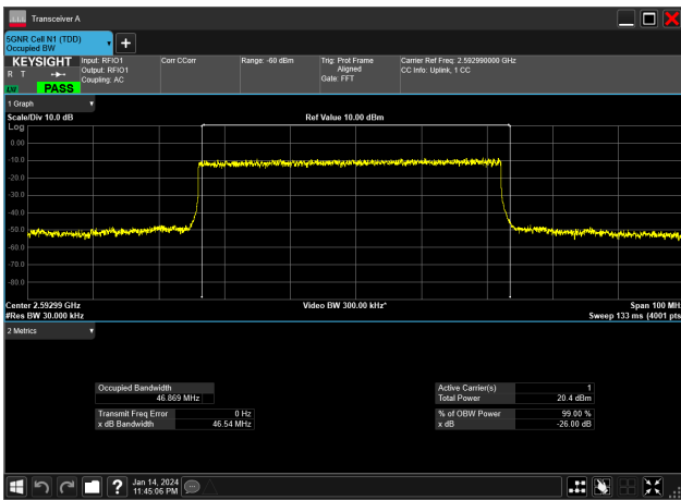
50MHz_30kHz_2592.99MHz_DFT-s-OFDM 64 QAM_RB128@0&46.869 MHz
