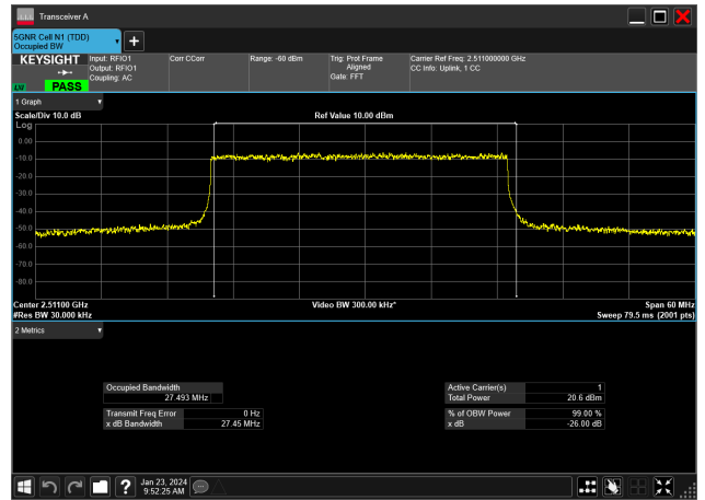
30MHz_30kHz_2511MHz_DFT-s-OFDM 16 QAM_RB75@0&27.493 MHz
