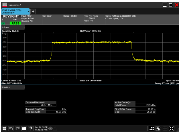
50MHz_30kHz_2592.99MHz_DFT-s-OFDM QPSK_RB128@0&46.971 MHz
