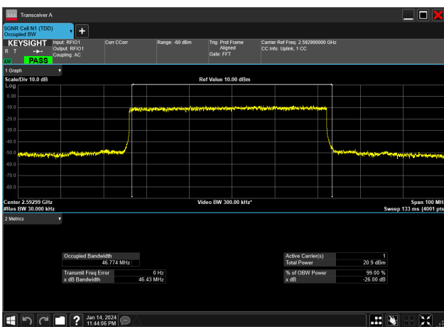
50MHz_30kHz_2592.99MHz_DFT-s-OFDM 16 QAM_RB128@0&46.774 MHz
