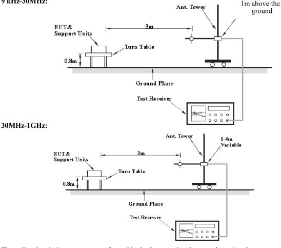
The radiated emission tests were performed in the 3-meter chamber test site, using the setup accordance with the ANSI C63.10-2013.
