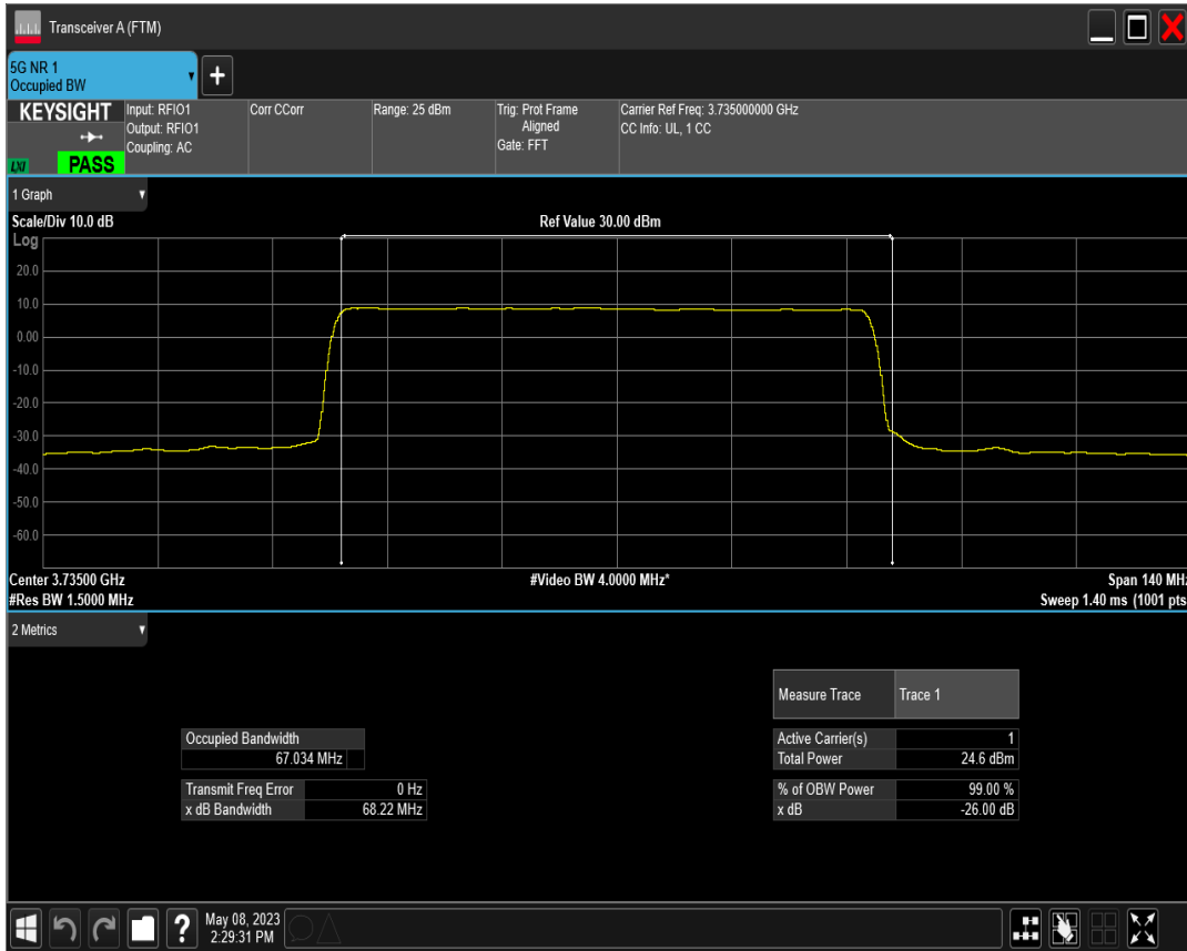
n78(3700-3800) SCS=30kHz DFT_QAM16 BW=70MHz Channel=649000 RB=180@0
