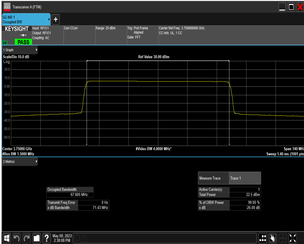
n78(3700-3800) SCS=30kHz DFT_BPSK BW=70MHz Channel=651000 RB=180@0
