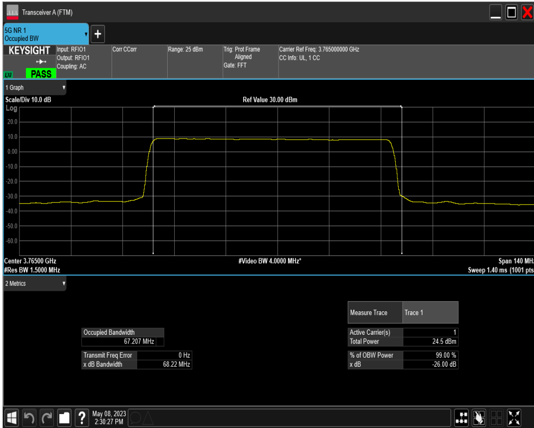
n78(3700-3800) SCS=30kHz DFT_QAM16 BW=70MHz Channel=651000 RB=180@0
