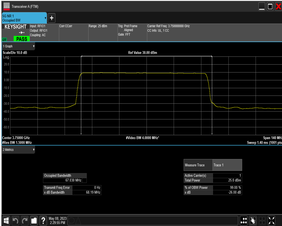
n78(3700-3800) SCS=30kHz DFT_QPSK BW=70MHz Channel=650000 RB=180@0
