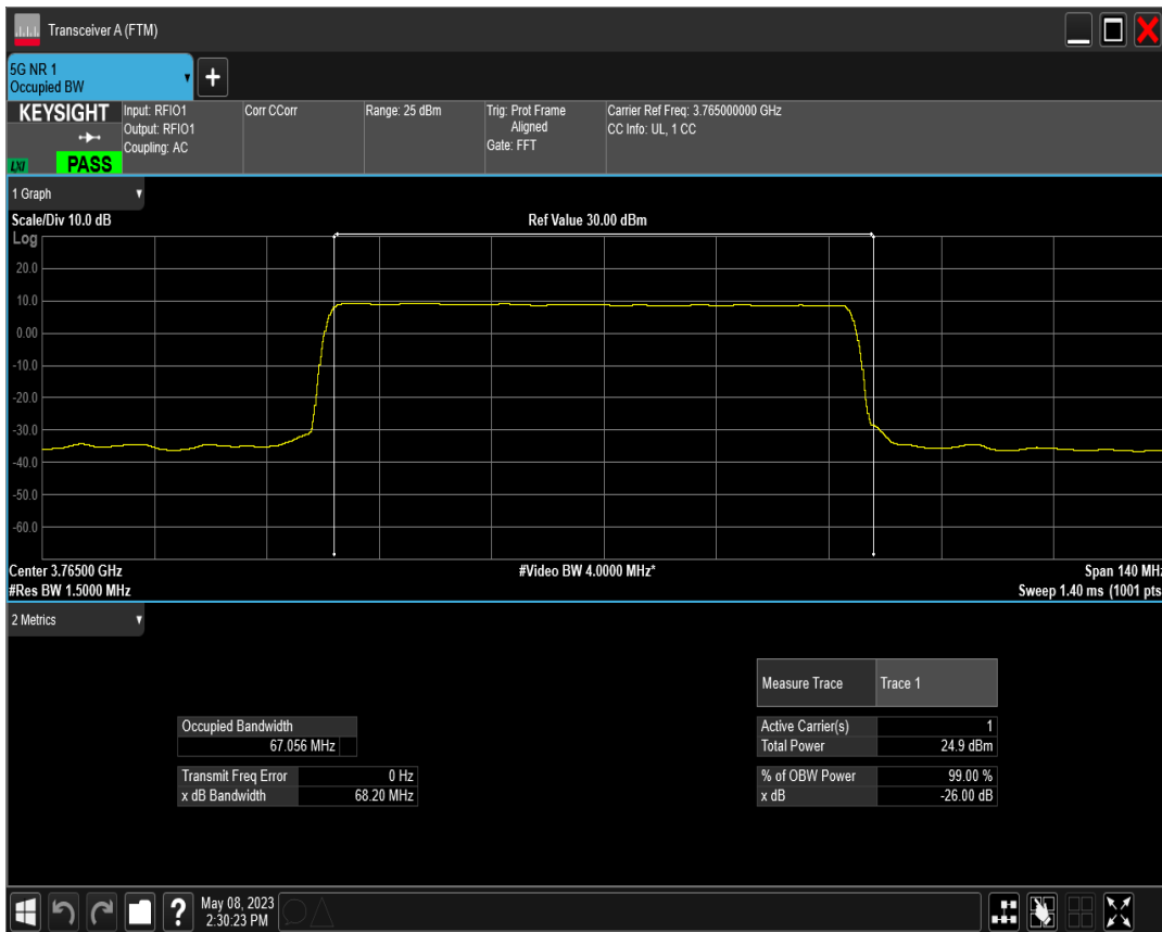
n78(3700-3800) SCS=30kHz DFT_QPSK BW=70MHz Channel=651000 RB=180@0
