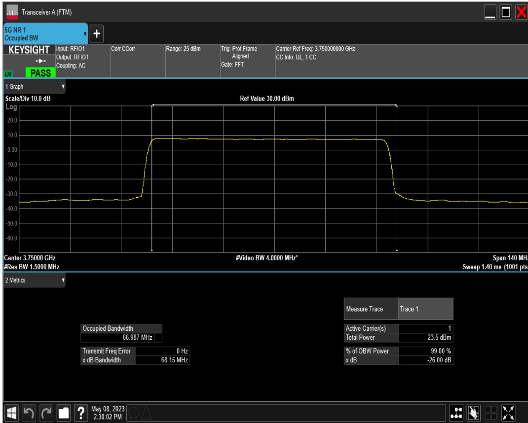
n78(3700-3800) SCS=30kHz DFT_QAM64 BW=70MHz Channel=650000 RB=180@0
