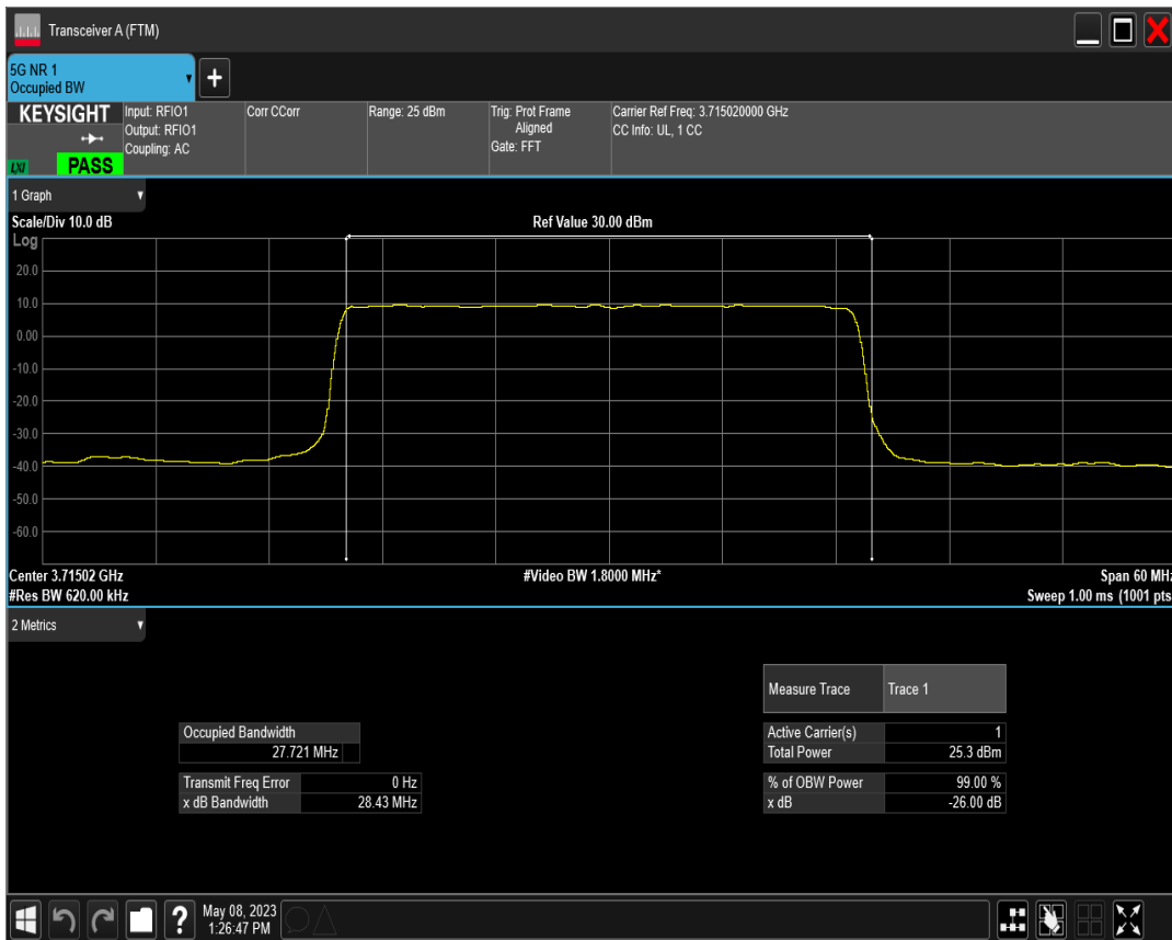
n77(3700-3980) SCS=30kHz DFT_QPSK BW=30MHz Channel=647668 RB=75@0
