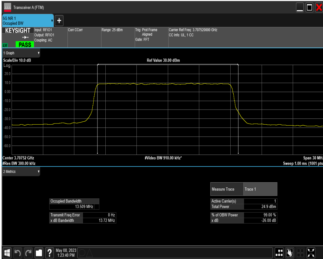
n77(3700-3980) SCS=30kHz DFT_QAM16 BW=15MHz Channel=647168 RB=36@0
