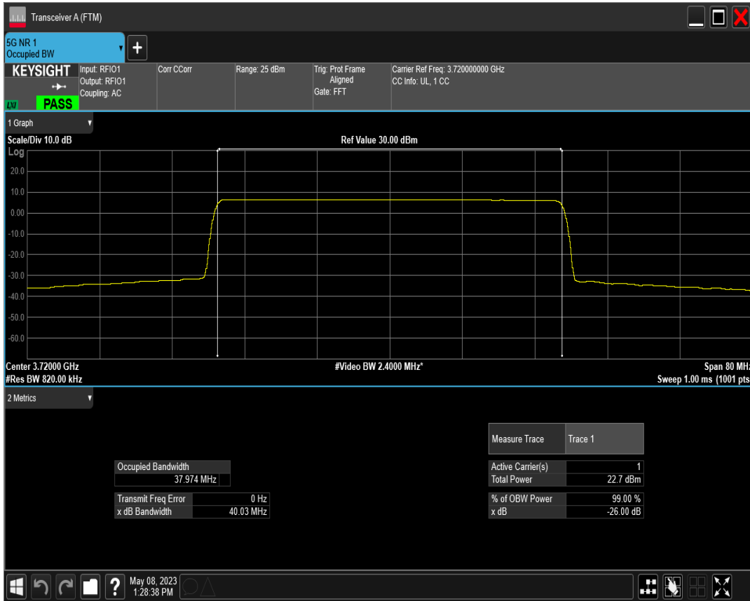
n77(3700-3980) SCS=30kHz DFT_BPSK BW=40MHz Channel=656000 RB=100@0
