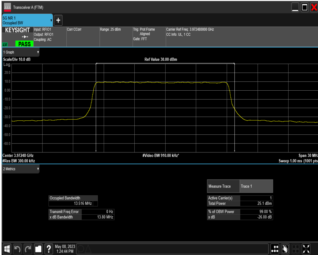
n77(3700-3980) SCS=30kHz DFT_QAM16 BW=15MHz Channel=664832 RB=36@0
