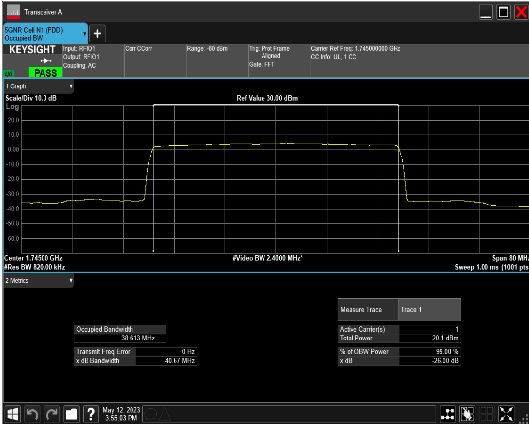
n66 SCS=15kHz DFT_QAM256 BW=40MHz Channel=349000 RB=216@0
