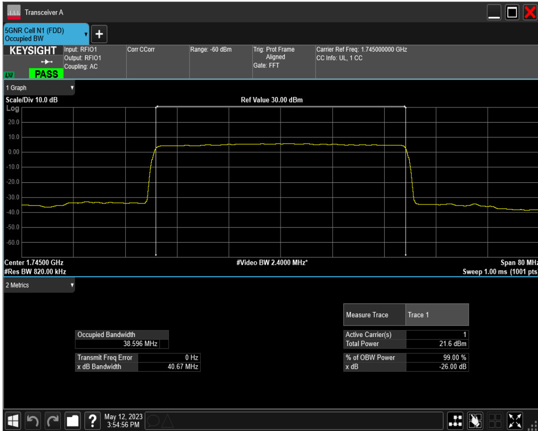
n66 SCS=15kHz DFT_QAM16 BW=40MHz Channel=349000 RB=216@0
