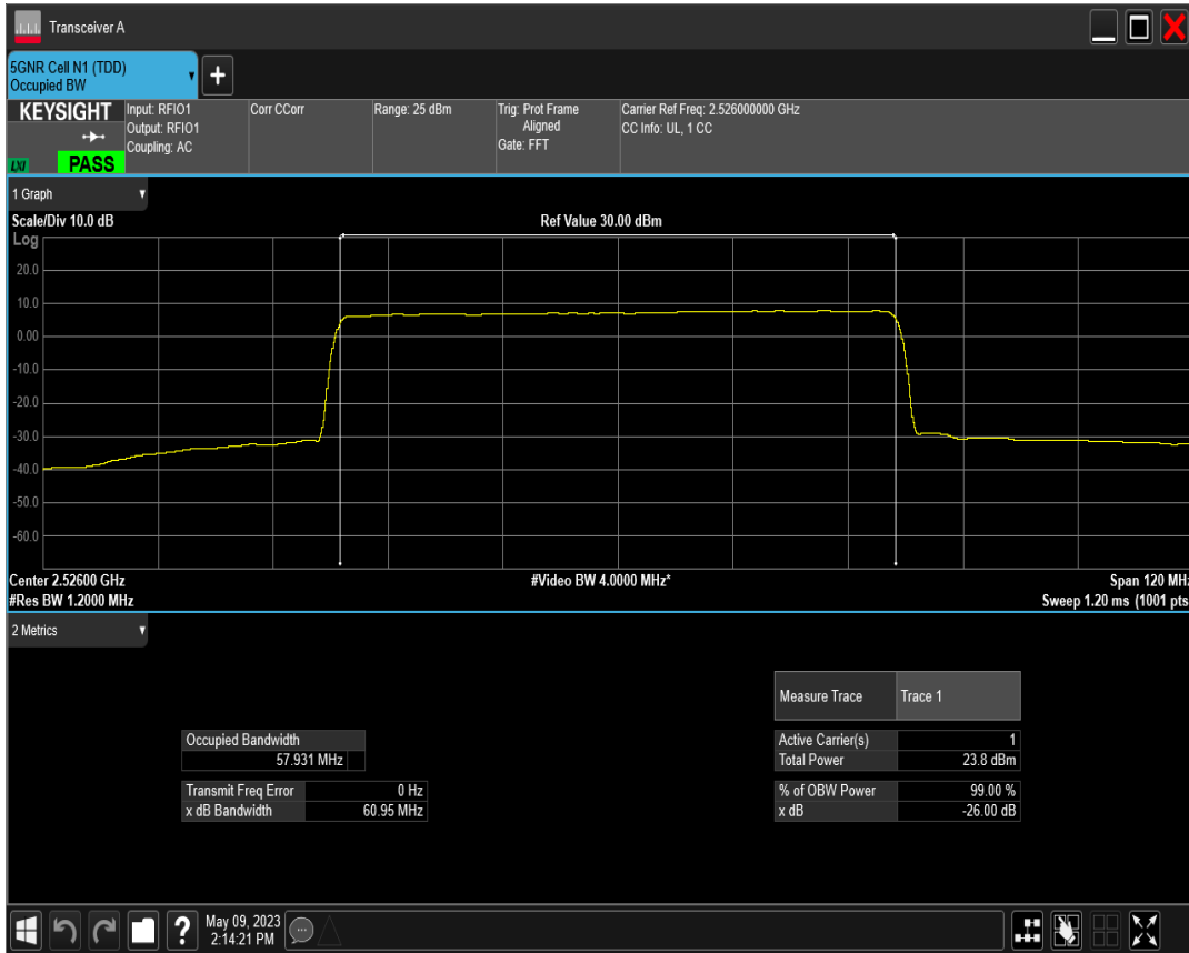
n41 SCS=30kHz DFT_QAM256 BW=60MHz Channel=505200 RB=162@0
