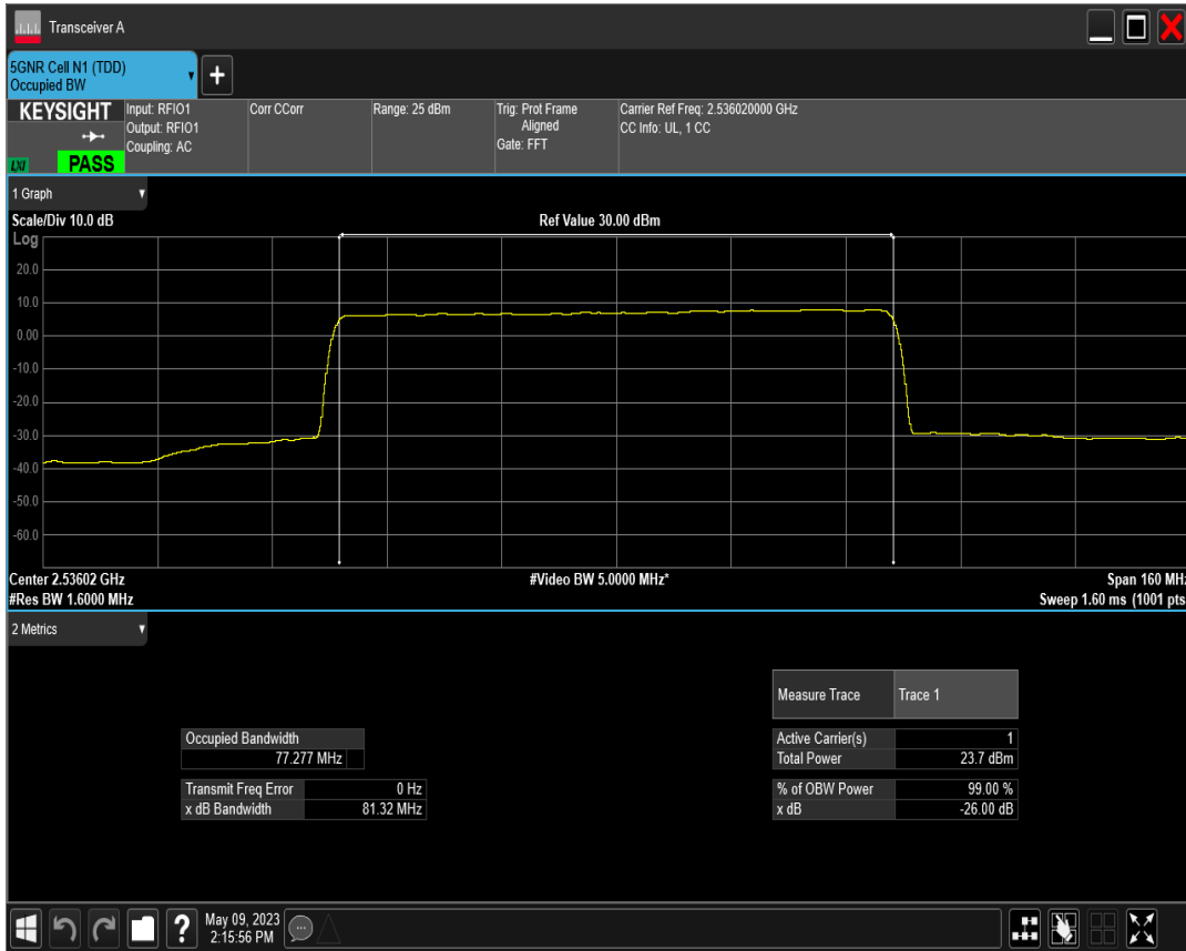
n41 SCS=30kHz DFT_QAM256 BW=80MHz Channel=507204 RB=216@0
