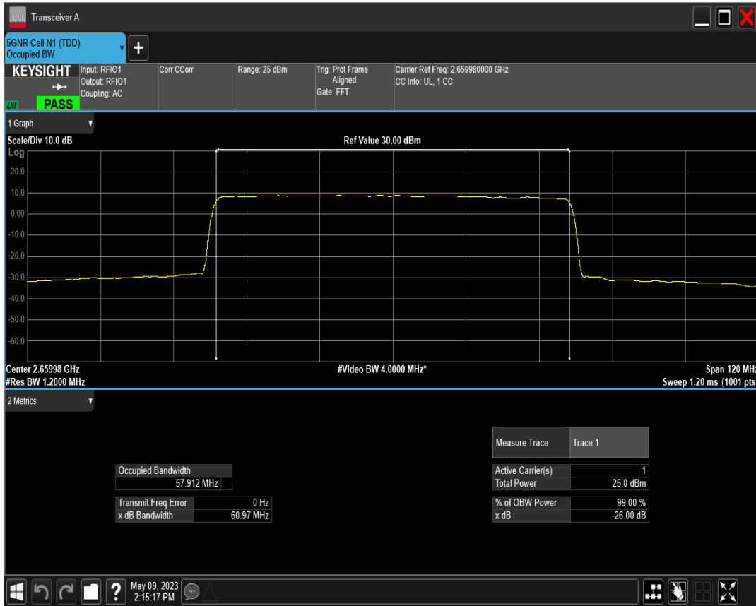
n41 SCS=30kHz DFT_QAM16 BW=60MHz Channel=531996 RB=162@0
