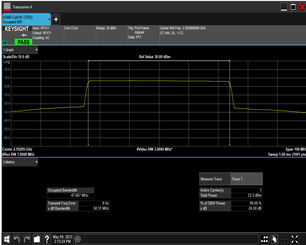
n41 SCS=30kHz DFT_BPSK BW=50MHz Channel=532998 RB=128@0
