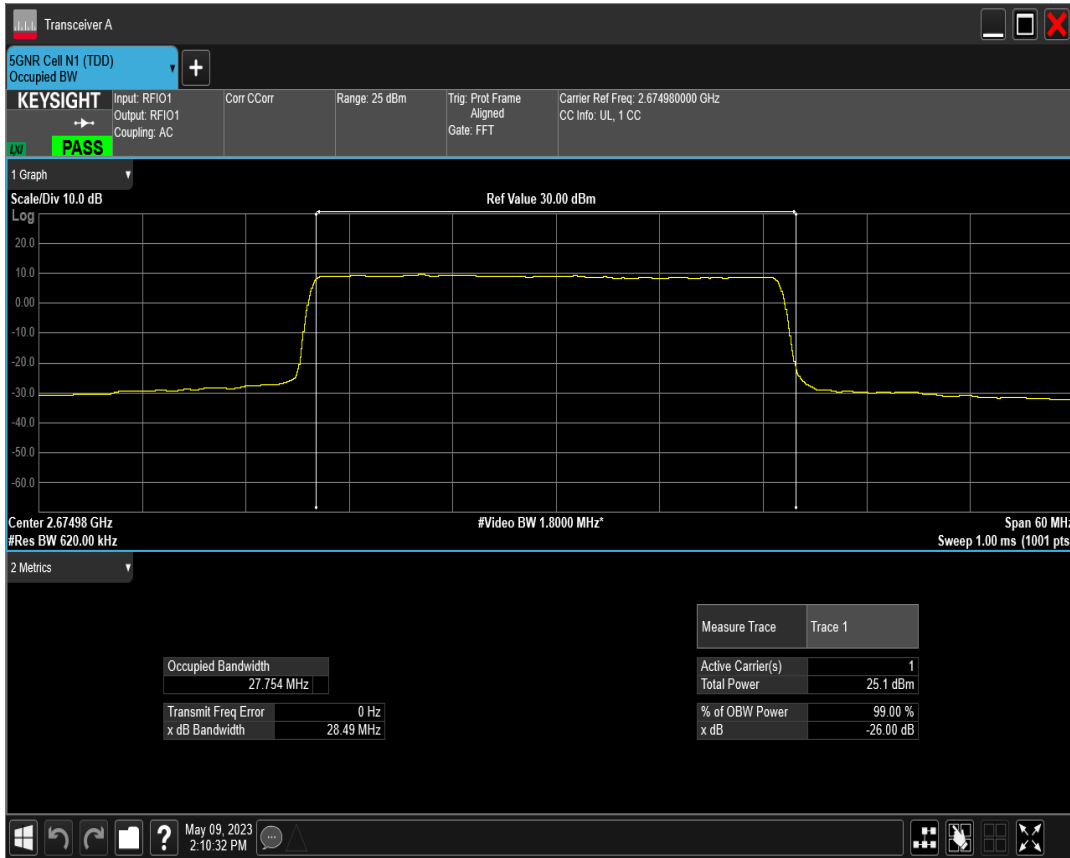
n41 SCS=30kHz DFT_QAM16 BW=30MHz Channel=534996 RB=75@0
