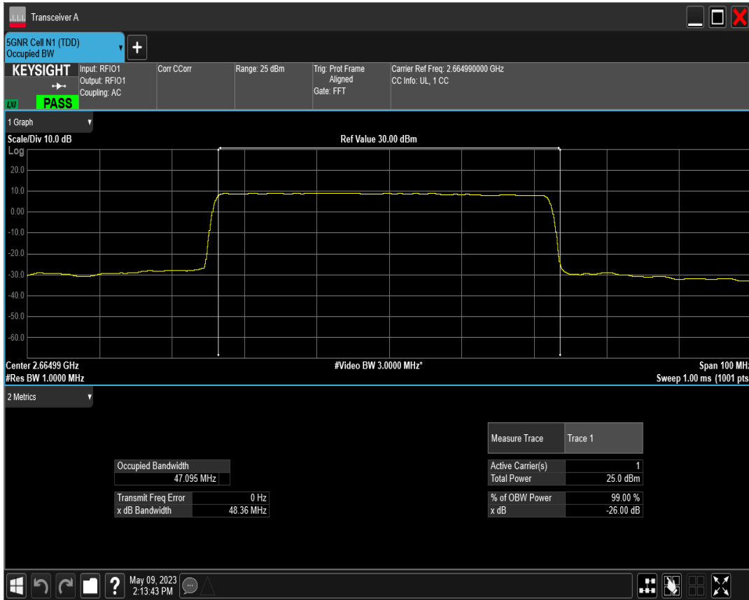
n41 SCS=30kHz DFT_QAM16 BW=50MHz Channel=532998 RB=128@0
