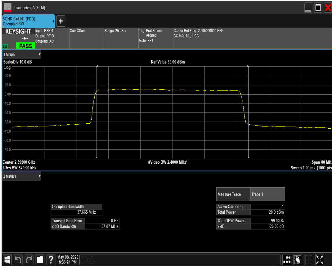
n38 SCS=30kHz DFT_QAM64 BW=40MHz Channel=519000 RB=100@0
