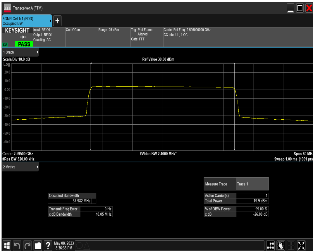
n38 SCS=30kHz DFT_BPSK BW=40MHz Channel=520000 RB=100@0
