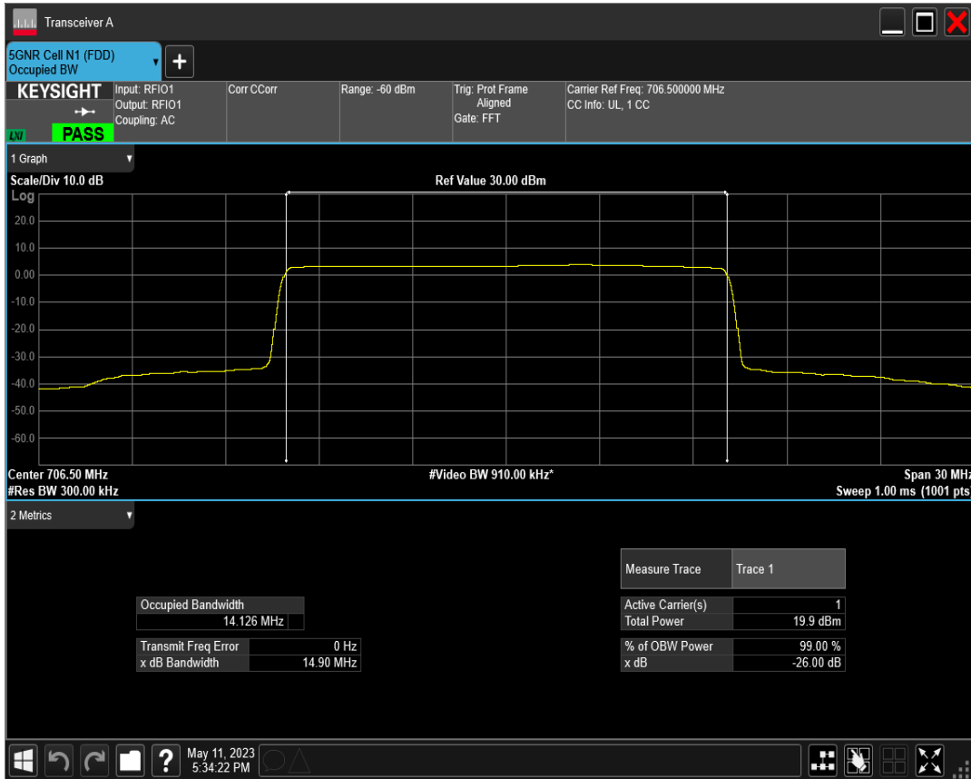
n12 SCS=15kHz DFT_BPSK BW=15MHz Channel=141500 RB=75@0
