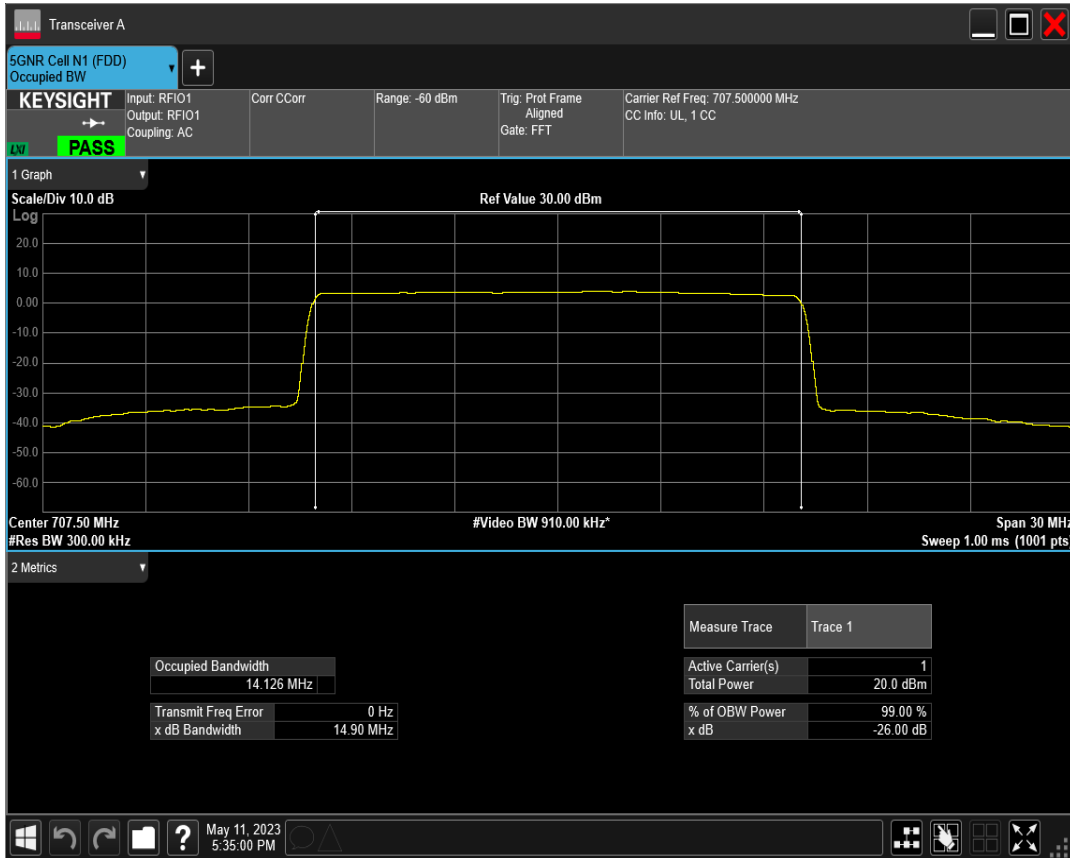
n12 SCS=15kHz DFT_BPSK BW=15MHz Channel=141700 RB=75@0
