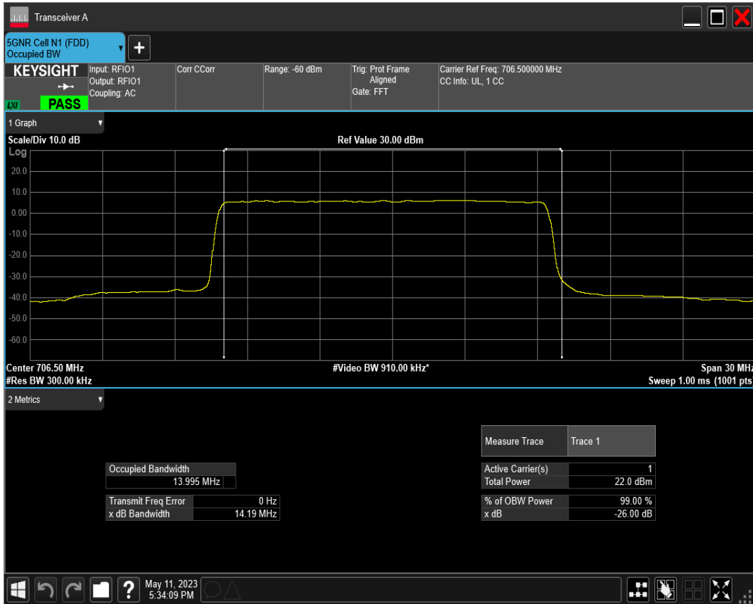
n12 SCS=15kHz DFT_QAM16 BW=15MHz Channel=141300 RB=75@0
