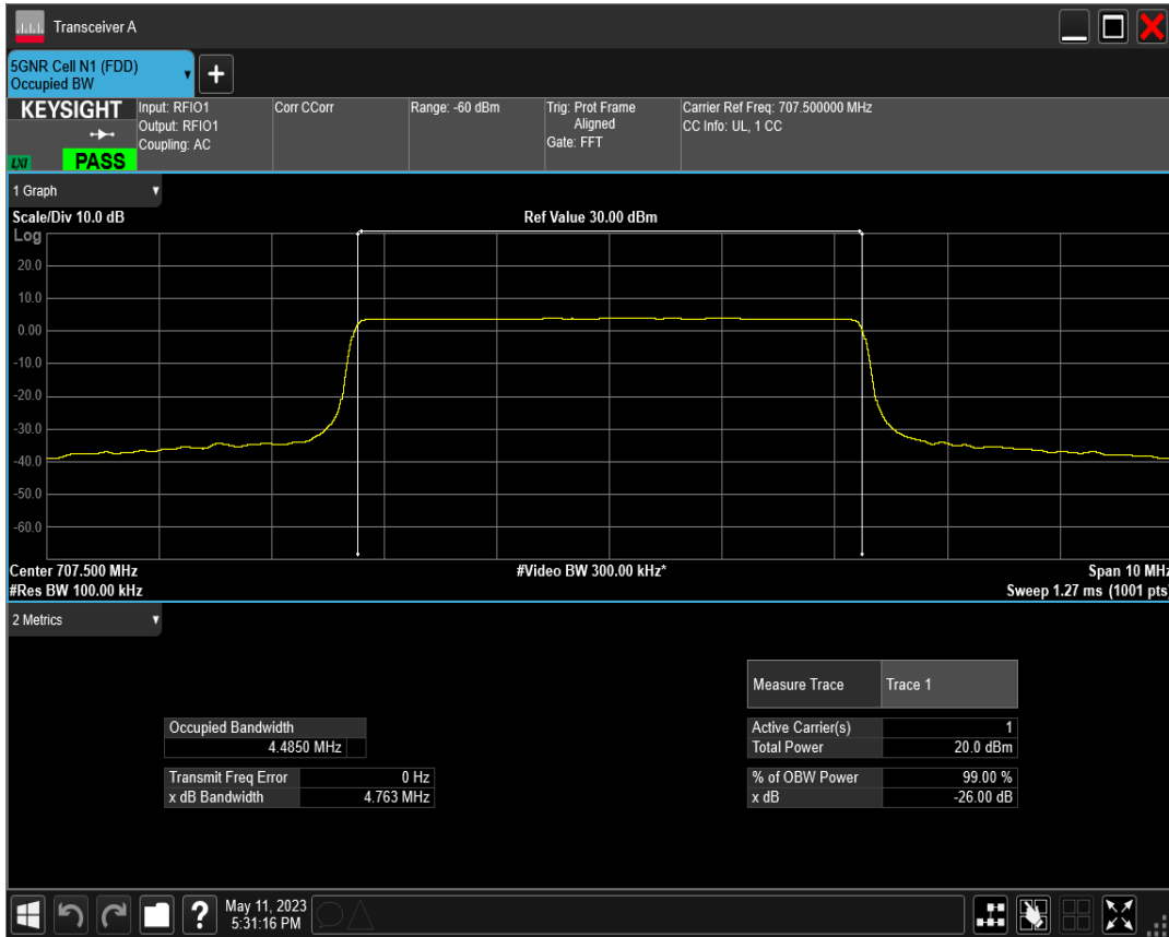
n12 SCS=15kHz DFT_BPSK BW=5MHz Channel=142700 RB=25@0
