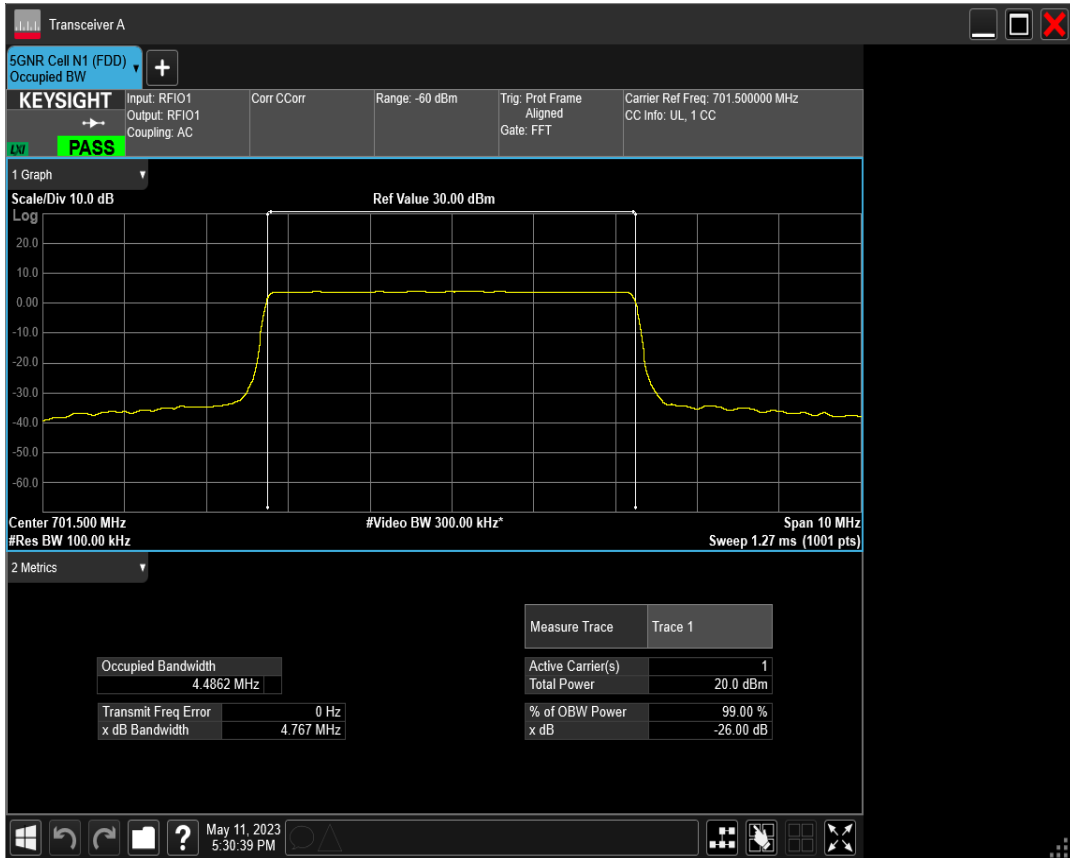
n12 SCS=15kHz DFT_BPSK BW=5MHz Channel=141500 RB=25@0
