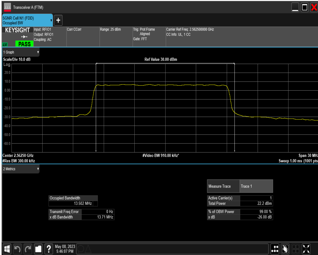
n7 SCS=30kHz DFT_QAM16 BW=15MHz Channel=512500 RB=36@0
