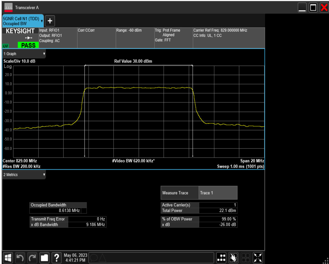
n5 SCS=30kHz DFT_QAM16 BW=10MHz Channel=165800 RB=24@0
