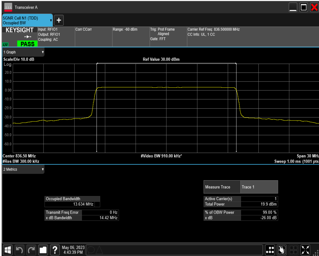
n5 SCS=30kHz DFT_BPSK BW=15MHz Channel=168300 RB=36@0
