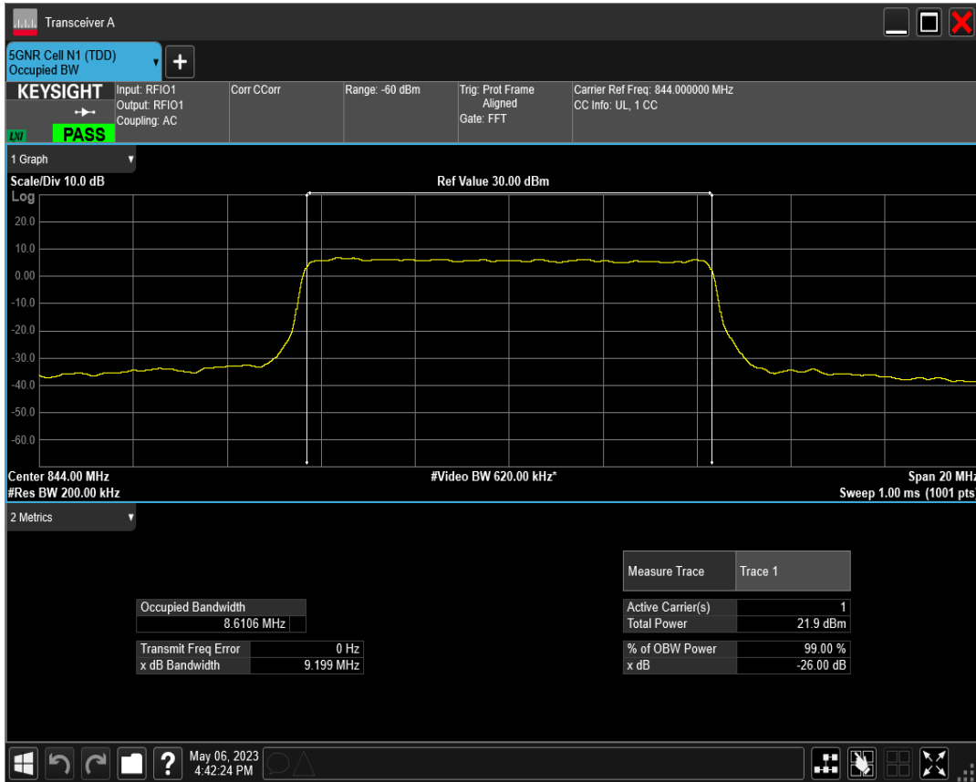
n5 SCS=30kHz DFT_QAM16 BW=10MHz Channel=168800 RB=24@0
