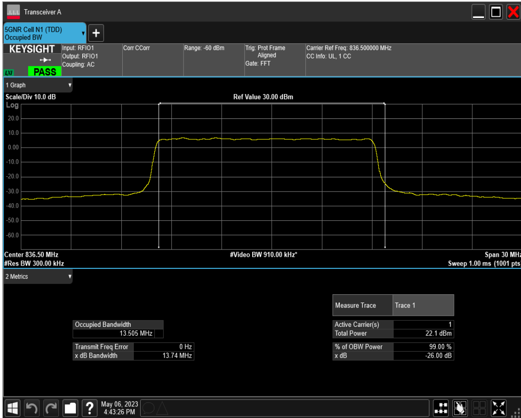
n5 SCS=30kHz DFT_QAM16 BW=15MHz Channel=167300 RB=36@0
