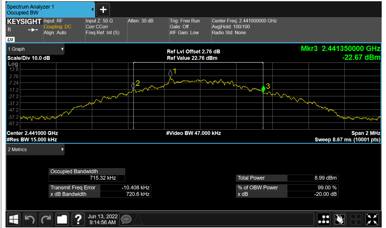
-20dB Bandwidth NVNT 1-DH1 2480MHz Ant1
